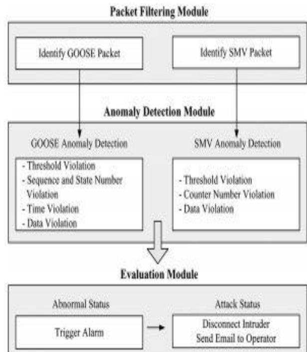
**Figure.1: Packet filtering internal Process**
