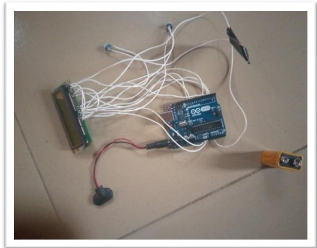
Fig. 2 (a) Arduino, LCD, and LM35 Temperature Sensor interfaced through wiring
